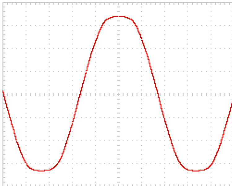
CLIPPING AT 40 WATTS / 4 OHMS
