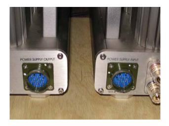
1. Locate the **Power Supply Output** (left) and **Power Supply Input** (right) on the rear panel. Both of them are male sockets.
